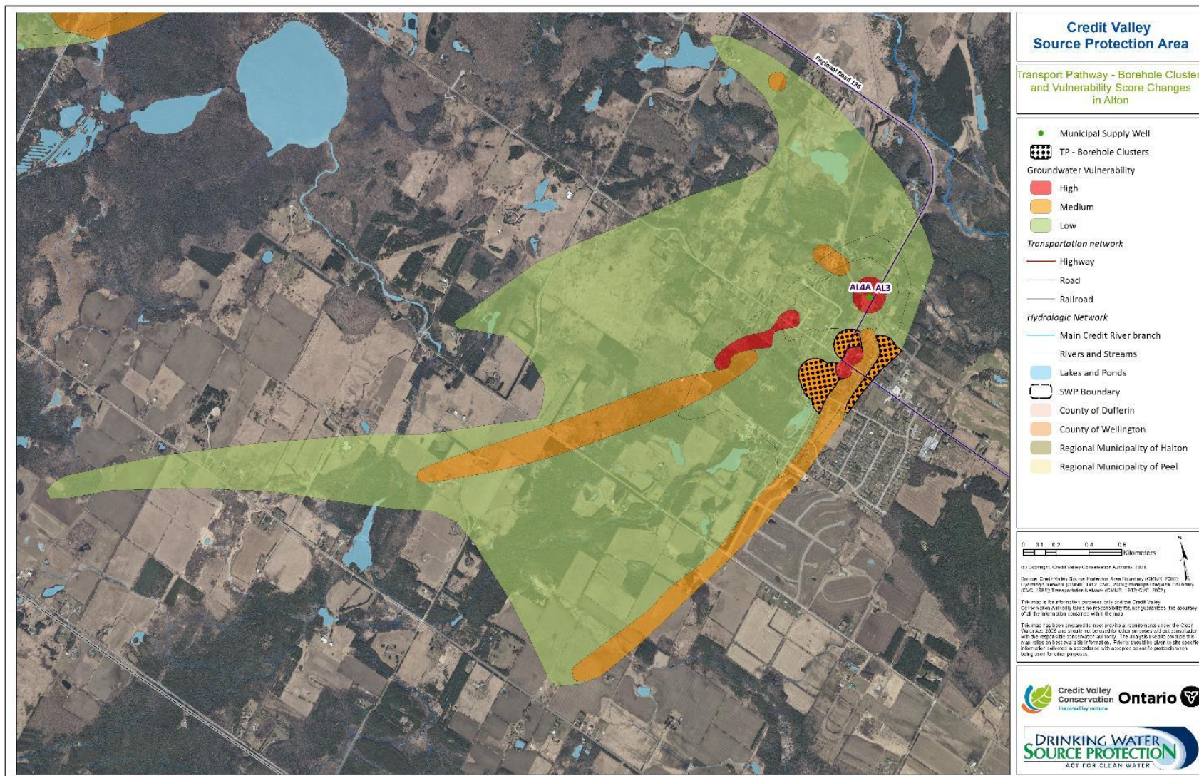
Figure 5: Transport Pathways related to wells and boreholes: Alton; recommended change in vulnerability rating – low to medium
