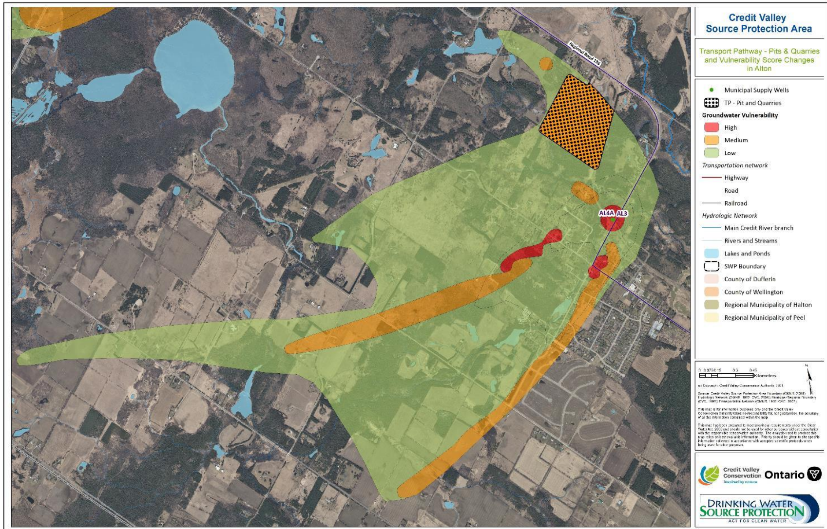
Figure 10: Transport Pathways related to aggregates: Alton; recommended change in vulnerability rating – low to medium
